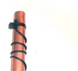
4) Wrap the electrical cable twice around the pipe;
