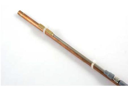
1) Place the sensor on the pipe, wrap and secure the cable ties around the two ends;
