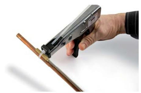
3) Use the tool to tighten and then cut the cable tie 1209874AXX;
